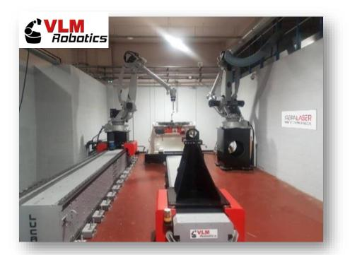
The large-size parts manufacturing cell delivered by VLM-Robotics is exemplary in its design since its **18 axes are driven by a unique Sinumerik 840D numerical control (NC)**. Its digital and multi-channel control architecture is also completed by the implementation of Direct Control, which consists of controlling the axis motors directly by the NC, making it possible to manage the precision and dynamics of the machine.
