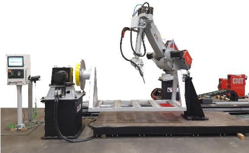
From 1 robot cells (part : 5m x 1,5m x 1,5 m) to 2 robots cells 18 axis for part up to 6 m x 3 m x 1,5 m and 3 tonnes
