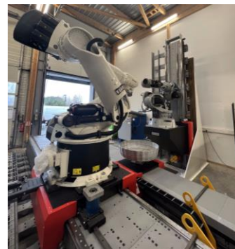
20-axis version with linear axis horizontal and vertical for one workpiece up to H: 5 m * Diam: 2 m
